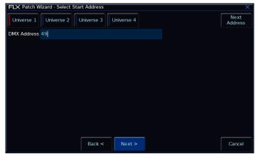
Figure 5 – Setting the DMX address
